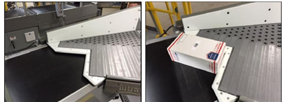
Source: United Sortation Solutions (USS) Operations Training Course Guide. The first photograph shows the template and the second shows the template with a package.
